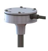
When installing the 9402, mount the sensor into the tank with the matching fitting. When installing into a metal threaded fitting or coupling, pipe sealant or appropriately rated PTFE tape is recommended to be used on the threads.
