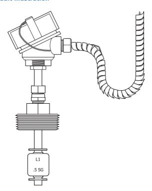
There are design options that can be considered to protect the sensor from moisture contaminating the internals of the sensor. One popular option is to select a cable for lead wires and a sealed "cord grip" to create a water tight seal at the end of the sensor. There are other options create a water tight sensor. Contact FPI Sensors to discuss your specific application requirements.
