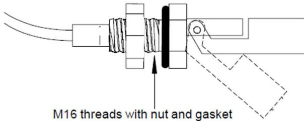
M16 threads with nut and gasket
